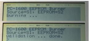
Special software flashes 32KB content prepared at slot 1 (e.g. on a CE-1600M) onto the EEPROM module.
