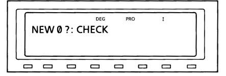
This message tells you that the computer recognizes the additional memory and is waiting for you to clear the memory area of any possible remaining spurious data. Note that this message comes up only when the memory modules are installed for expansion memory. The message is not displayed if a program module is configured as a RAM disk or program memory. Use of the modules is described in PART III of this manual.
